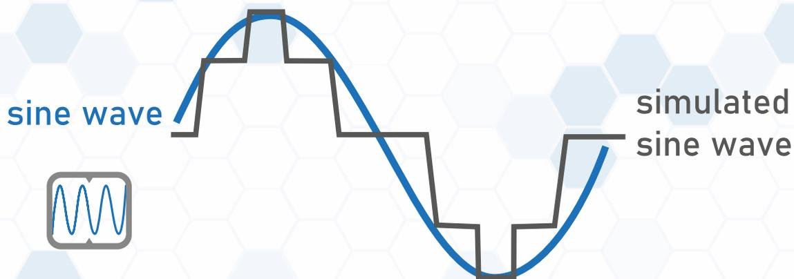
The **Pure Sine Wave** feature comes in handy when **sensitive equipment** is connected to the UPS. Sensitive equipment can range from a motor-based load to a home record player. Typical applications for pure sine wave UPS systems involve the **protection** of critical server, network, medical and telecommunications equipment or electronic equipment that is particularly sensitive to input power, such as lab test equipment.
