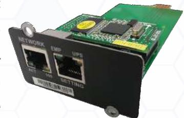
The **Modbus Card** is a communication accessory that provides a pair of RJ-45 Interface for remote monitoring and controlling of the UPSs. It converts standard RS232 signal to RS232 signal with a specified address, which allows to control many UPSs from one computer.
