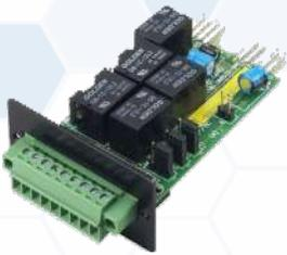
**AS/400 Cards** provide potential free connection pins (dry contacts) for remote shutdown and monitoring of the UPS. It is frequently used along with PLCs and signal control panels. Information delivered can be triggered by UPS failure, alarm, main fail, bypass, battery low, UPS on. By using a AS/400 it is possible to shutdown the UPS remotely.
